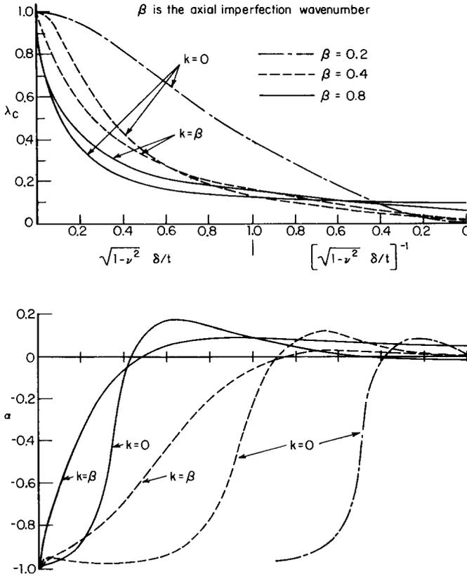
FIG. 2. Buckling and postbuckling of unstiffened cylindrical shell.
