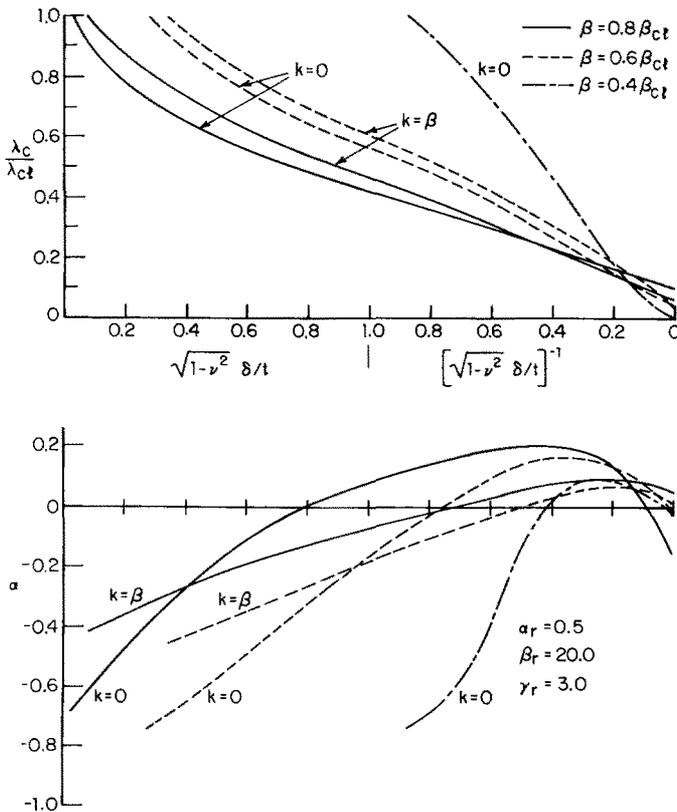
FIG. 4. Buckling and postbuckling of stiffened cylindrical shell.
