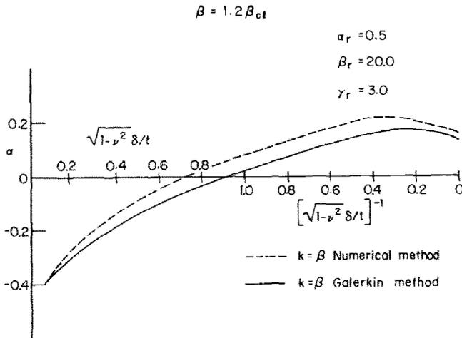
FIG. 6. Postbuckling behavior predicted by the Galerkin method.
