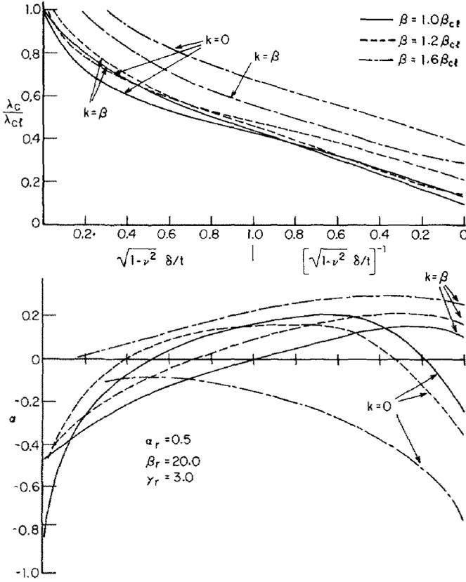
FIG. 5. Buckling and postbuckling of stiffened cylindrical shell.
