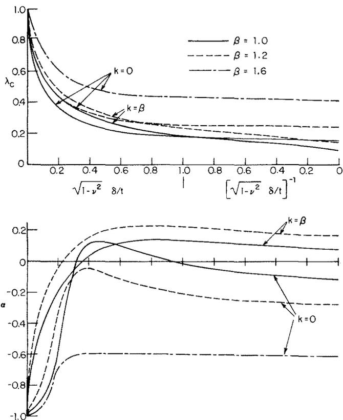
FIG. 3. Buckling and postbuckling of unstiffened cylindrical shell.
