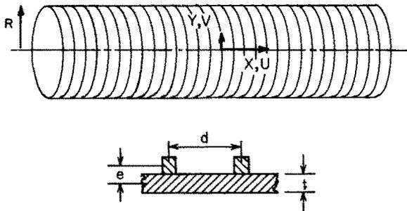
FIG. 1. Part of ring stiffened cylindrical shell.
